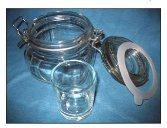
500 ml capacity clamp-lid glass **receiver** container, <u>silicone</u> lid-to-jar **gasket**, and 90 ml capacity **reactor** glass candle holder. **Reactor** is 2" (5 cm) diameter, 2.5" (6.35 cm) tall.
