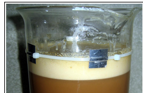
LET Vitamin-C in Ultrasonic Cleaner - water temp is 32C (90F)
