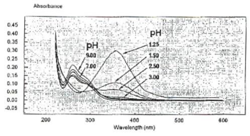
UV-Vis absorption spectra showing the release of ClO<sub>2</sub> from sodium chlorite (buffered in the form of "stabilized chlorine dioxide") at various pH values. Readings were taken after 60 minutes at ambient temperature. The initial chlorite concentration was 112 ppm. Notice the loss of chlorite at 262 nm as the pH is lowered, with the gain of ClO<sub>2</sub> at 360 nm. There is no release of ClO<sub>2</sub> above pH 3. from Multicomponent Spectroscopic Invetigations of Salivary Antioxidant,
