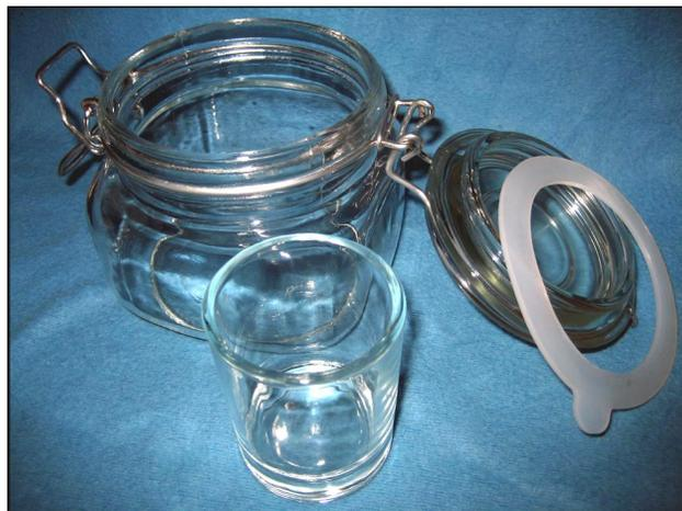
500 ml capacity clamp-lid glass **receiver** container, silicone lid-to-jar **gasket**, and 90 ml capacity **reactor** glass candle holder. **Reactor** is 2" (5 cm) diameter, 2.5" (6.35 cm) tall.
